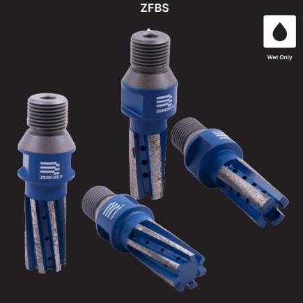
The ZENESIS<sup>™</sup> Finger Bits excel in CNC performance across stone materials, delivering precise, quiet, chip-free cutting at increased speeds. They accommodate soft to medium-hard materials (4 segments) or medium to hard ones (7 segments). The enhanced design utilizes our most advanced diamond pattern to date, which increases durability and prevents premature wear to ensure long tool life.
